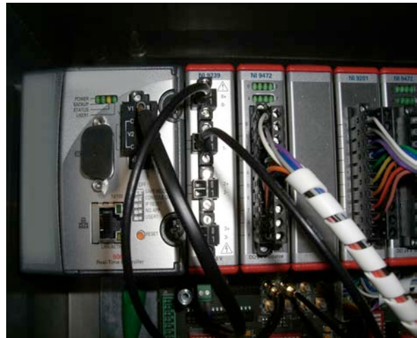
E-GOMS II - Controller (left hand) and the in- and output modules
