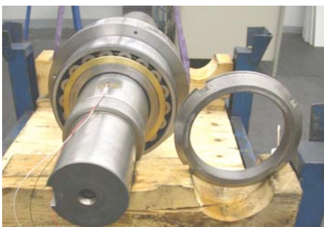
Strain gauges on the high speed shaft.
